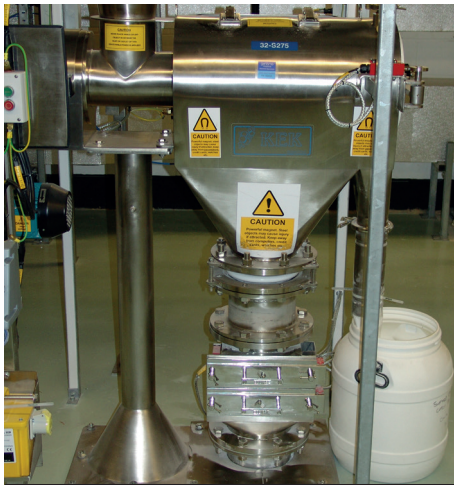
Pharmaceutical specification double row housed easy clean grid, pre and post sifter protection.
